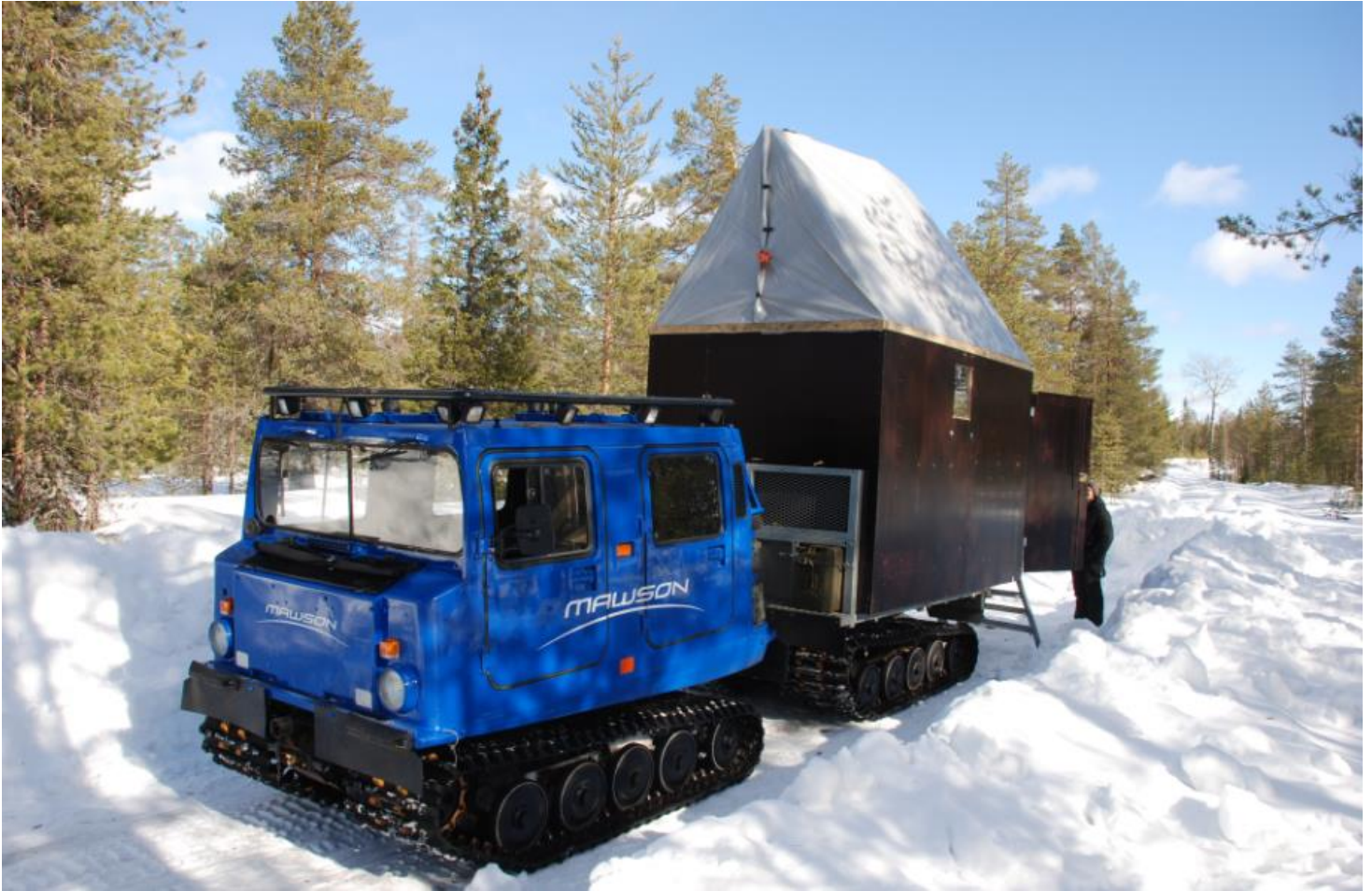
Photo 1: Mawson in-house diamond drill rig, mounted on an all-terrain bandwagon.
