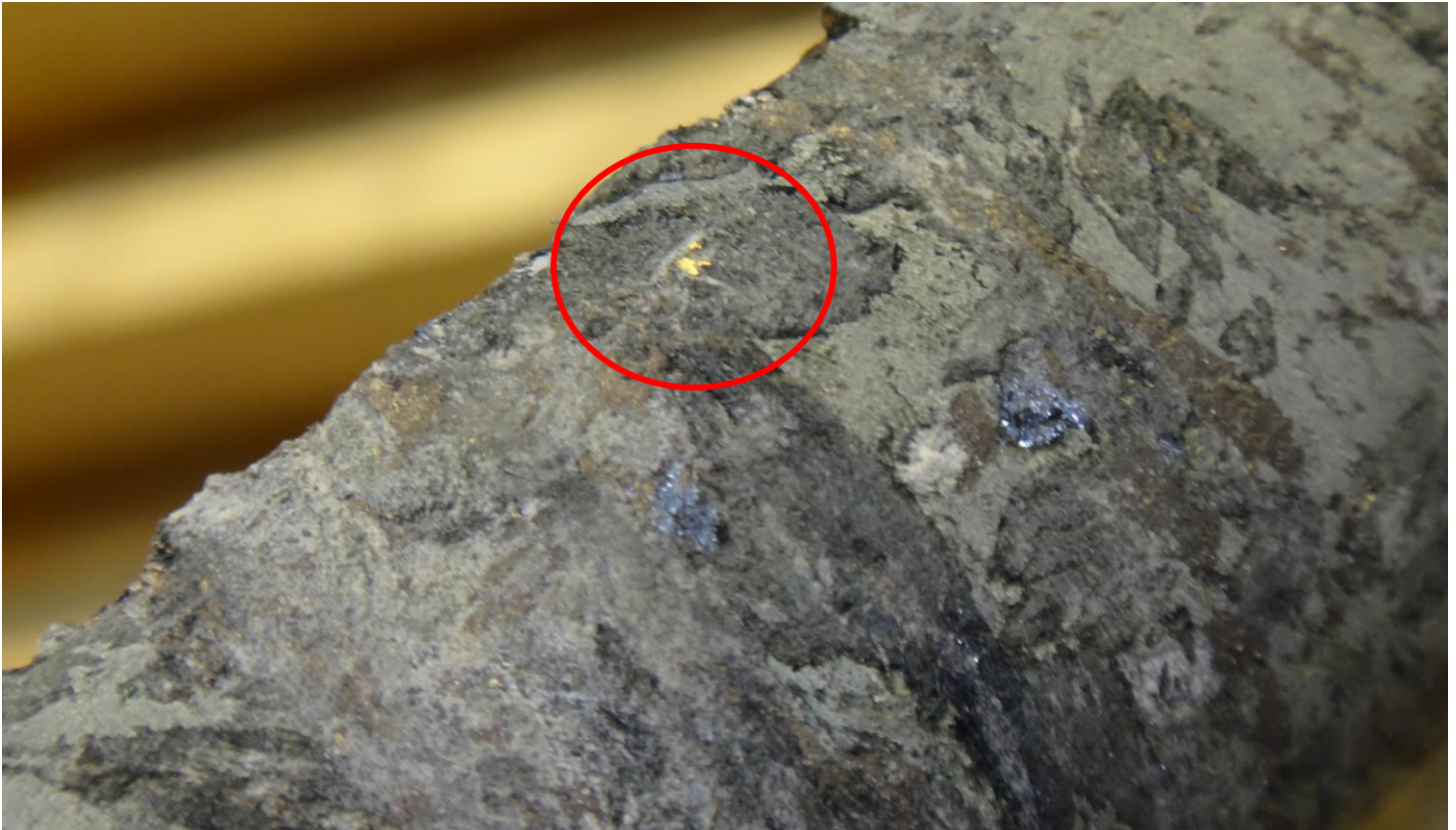
Figure 1: Visible gold in Drill hole PRAJ0107 at 28.95 metres (red circle) in chlorite-tourmaline-pyrrhotite rock. Drill core width approximately 25 mm.
