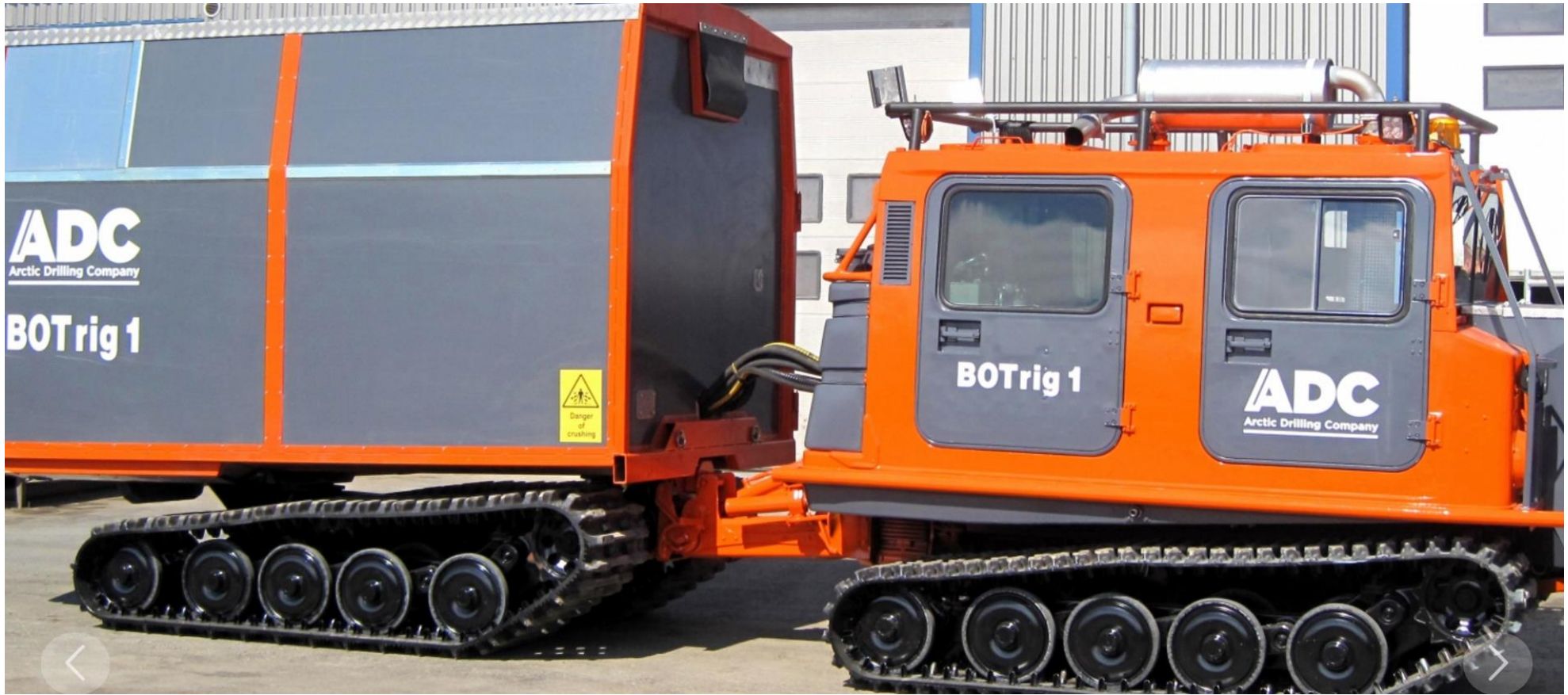
Figure 3: Base of Till ("BOT") percussion drill rig with a flow-through bit for glacial till geochemical sampling. Note the vehicle and trailer mounted on wide tracks to reduce impact on vegetation.
