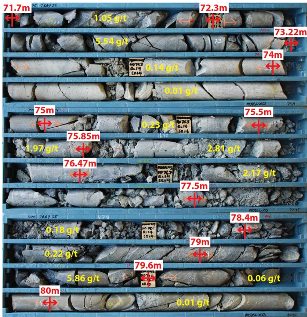
Figure 3: Drillhole MDDSC002 annotated HQ drill core (63.5mm diameter) showing downhole depth and gold grades.
