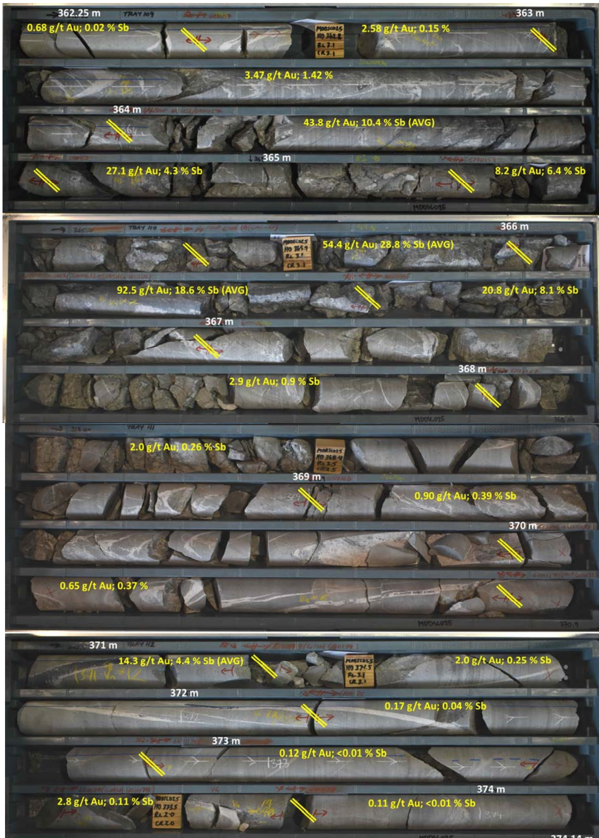
Figure 3: Annotated HQ drill core (63.5mm diameter) showing downhole depth and gold grades from MDDSC0025: 11.7 metres @ 12.4 g/t Au and 3.6 % Sb (16.0 g/t AuEq) from 362.0 metres in hole MDDSC025, including 3.0 metres @ 41.4 g/t Au and 12.0 % Sb (53.4 g/t AuEq) from 364.0 metres or 6.5 metres @ 20.6 g/t Au and 6.0 % Sb (26.6 g/t AuEq) from 362.5 metres and 0.5 metres @ 14.3 g/t Au and 4.4 % Sb (18.7 g/t AuEq) from 370.8 metres.
