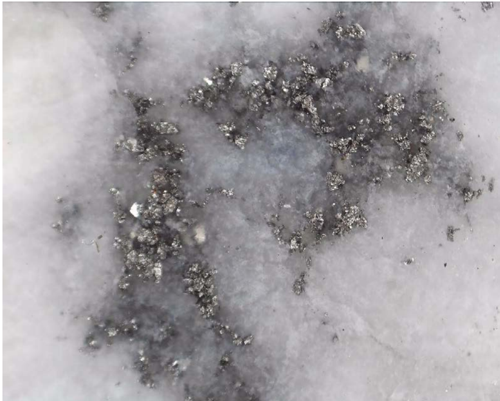
Photo 4: SDDSC050 713.9 m showing fine visible gold associated with arsenopyrite within quartz carbonate vein. Field of view 7 mm.
