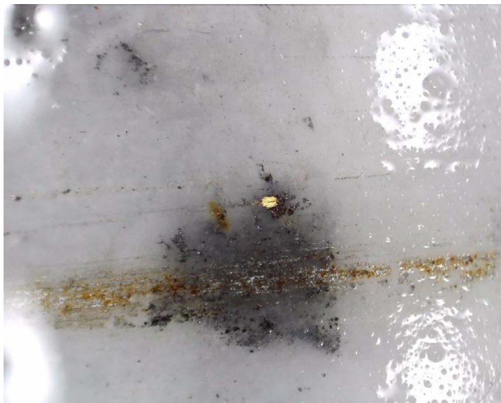
Photo 2: SDDSC050 713.9 m showing visible gold associated with and adjacent to pyrite veinlets within quartz carbonate vein. Field of view 7 mm.
