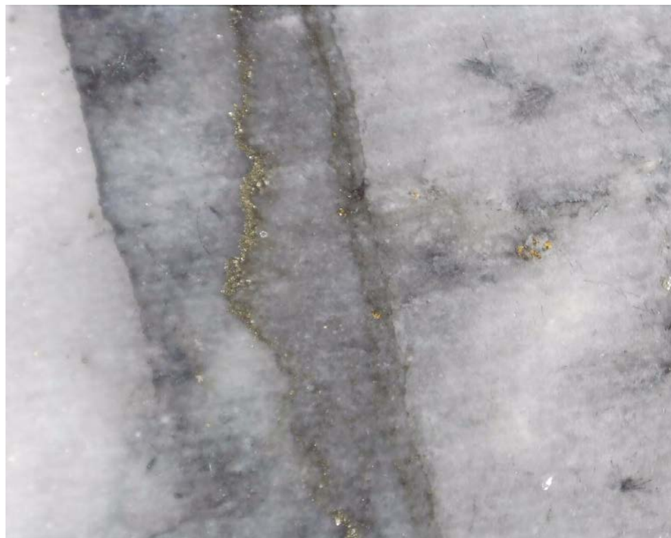
Photo 2: SDDSC050 713.9 m showing visible gold associated with and adjacent to pyrite veinlets within quartz carbonate vein. Field of view 7 mm.
