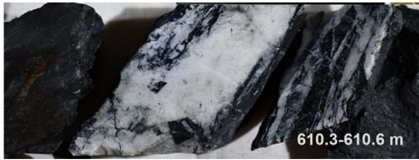
Photo 1: Quartz-carbonate-chlorite-graphite veined within zone of sericite-pyrite-chlorite alteration (from sample interval 610.3-610.6 metres).
