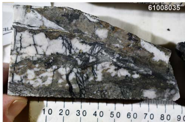
Photo 4: Fracture-controlled biotite-sericite-pyrite alteration with trace chalcopyrite associated with quartz-carbonate veining from sample interval 832.1-832.5 metres (0.22 wt % Cu).
