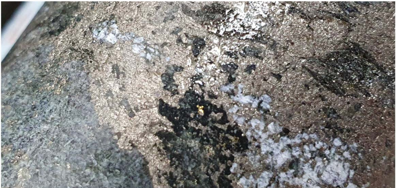
Photo 2: PAL0242 at 155.9 metres showing visible gold grain. The interval from 155.0-156.0 metres (1.0 metres length) assayed 26.0 g/t gold. Scale of core is NQ2 (50.7 mm diameter).
