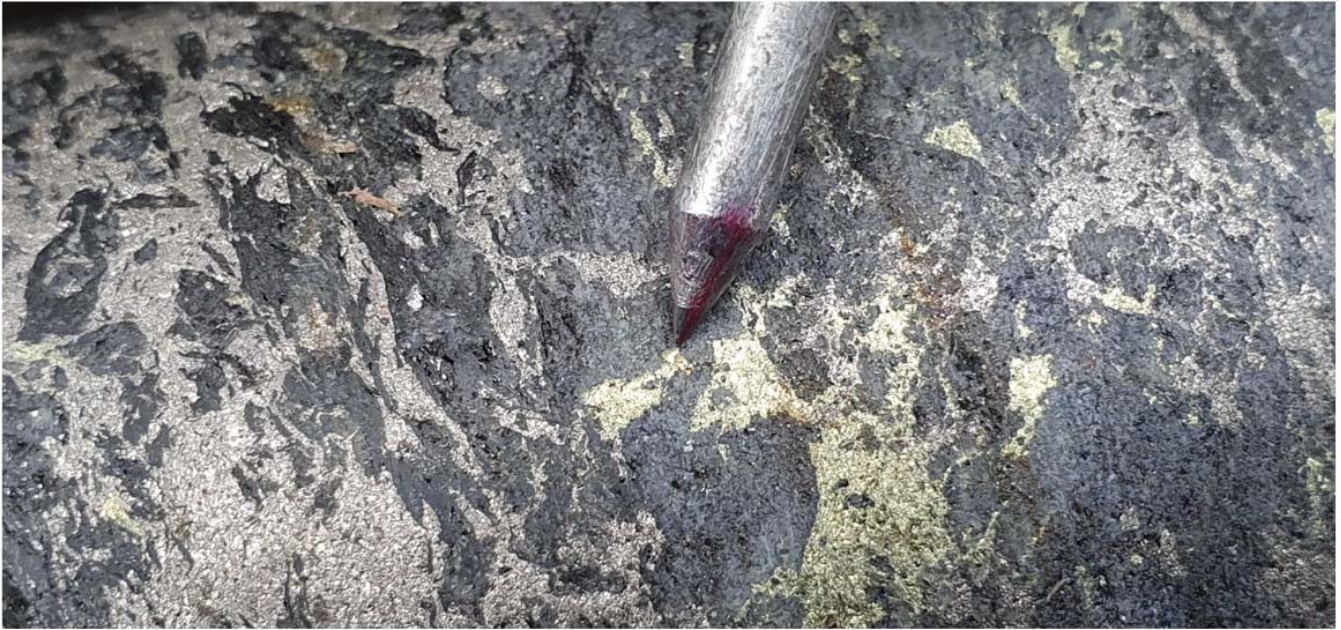
Photo 1: PAL0242 at 155.5 metres showing visible gold grain. The interval from 155.0-156.0 metres (1.0 metres length) assayed 26.0 g/t gold. Scale of core is NQ2 (50.7 mm diameter).
