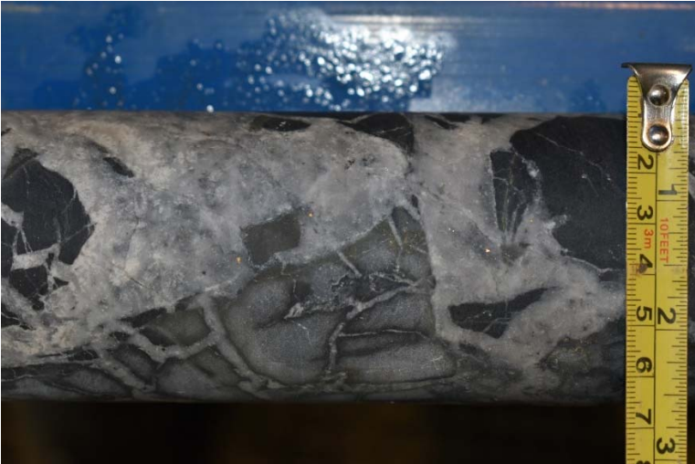
Photos 1,2, 3: Selected quartz carbonate veining and stockwork zone with abundant visible gold from 199.0-199.4 m (assayed 380.3g/t Au and 0.24% Sb) in drillhole SDDSC046 from the Rising Sun shoot. Brecciated gold-mineralized wall rocks are healed by quartz-carbonate veining and commonly have a halo of disseminated arsenopyrite and pyrite in the walls, extending for up to 50 cm beyond the veins. This is similar to other epizonal deposits such as Fosterville.
