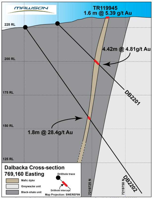
Figure 4: Geological cross-section of drilling intercepts from hole DB2201 & DB2202.
