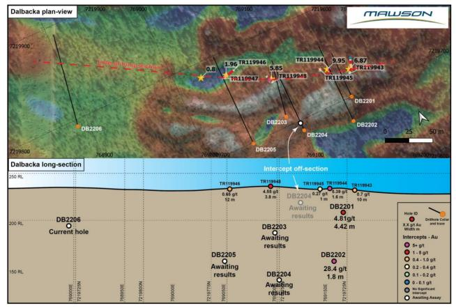
Figure 3: Geological long-section of drilling intercepts
