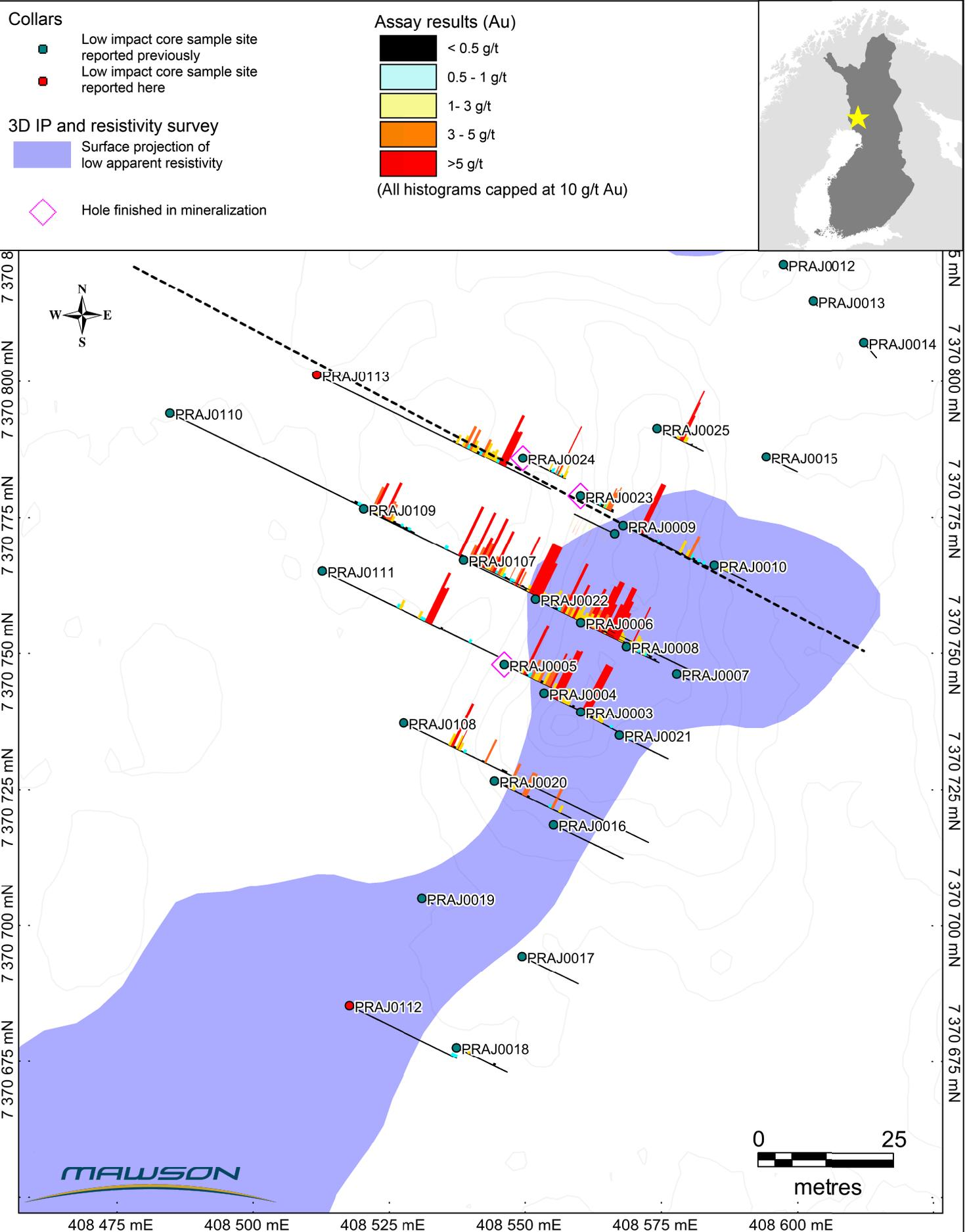
Figure 2: Section N7373 838 showing new results from drill hole PRAJ0113
