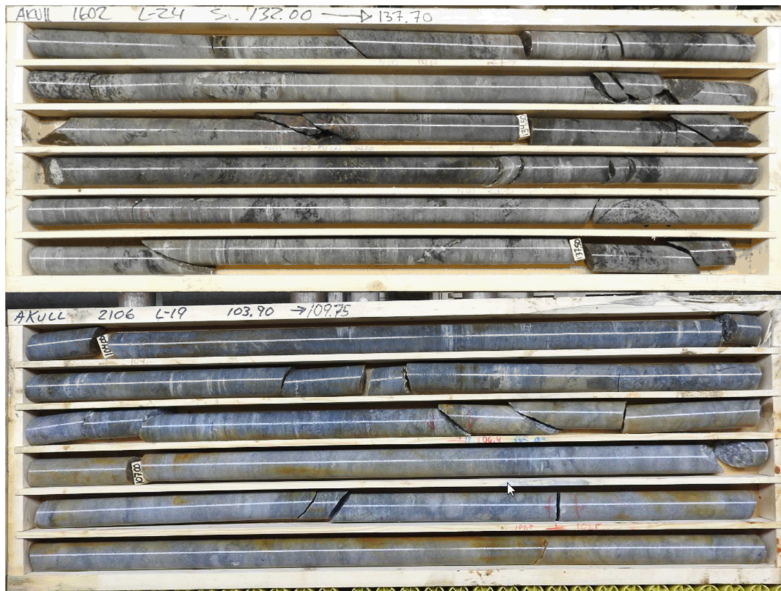
Figure 16: High-grade gold intersections, which are typical boxes of Kankberg mineralised core. Hole ID, box number and from-to depths are shown.
