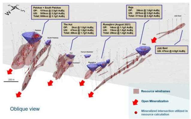
Figure 1: The <u>August 2021</u> open pit and underground constrained Rajapalot inferred mineral resource. Refer Mineral Resource Estimate NI 43-101 Technical Report, Rajapalot Finland, August 26, 2022.
