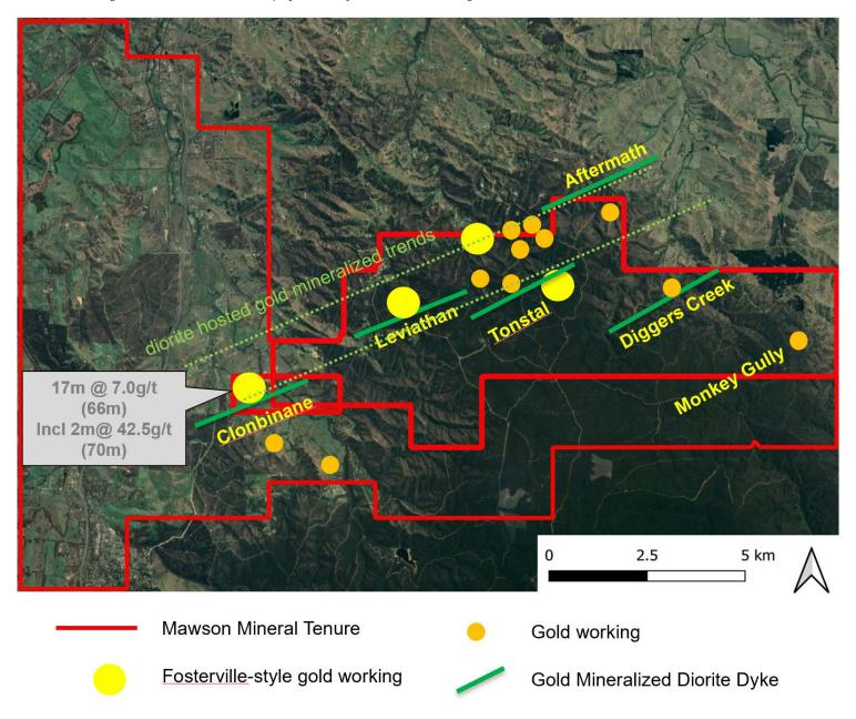
Figure 3: Drill plan of the Clonbinane drilled area showing the best results from two small drill campaigns in 1994 and 2008 that tested the system to 40-100 metres vertical depth over an 800 metre strike. Gold mineralization is located within, or proximal to, the dykes with mineralization continuing along structures that extend into the sedimentary country rock with gradually diminishing grades. (modified after Beadall 2008).
