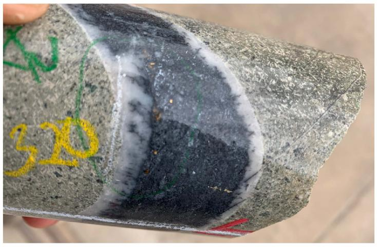
Photo 2: Drillhole MDDSC005 annotated HQ drill core (63.5 mm diameter) showing downhole depth and gold grades. Gold grades may slightly vary from those quoted in tables as laboratory assay repeats have been averaged during length weighted average calculations.
