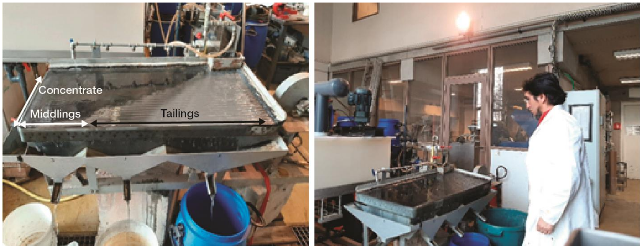
Figure 15. Photographs of the shaking table test work.
